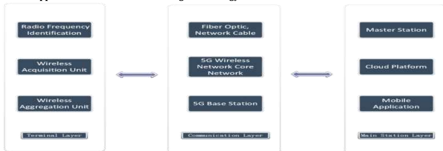
Figure 4. Network extension graph based on 5G
