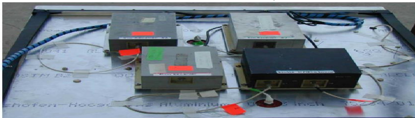
Figure 2. Several samples of microwave radiometers with a wavelength of 2.25, 6, 18/21 and 30 cm, were produced by a special design office of the Kotelnikov Institute of Radioengineering and Electronics RAS [10–12] .
