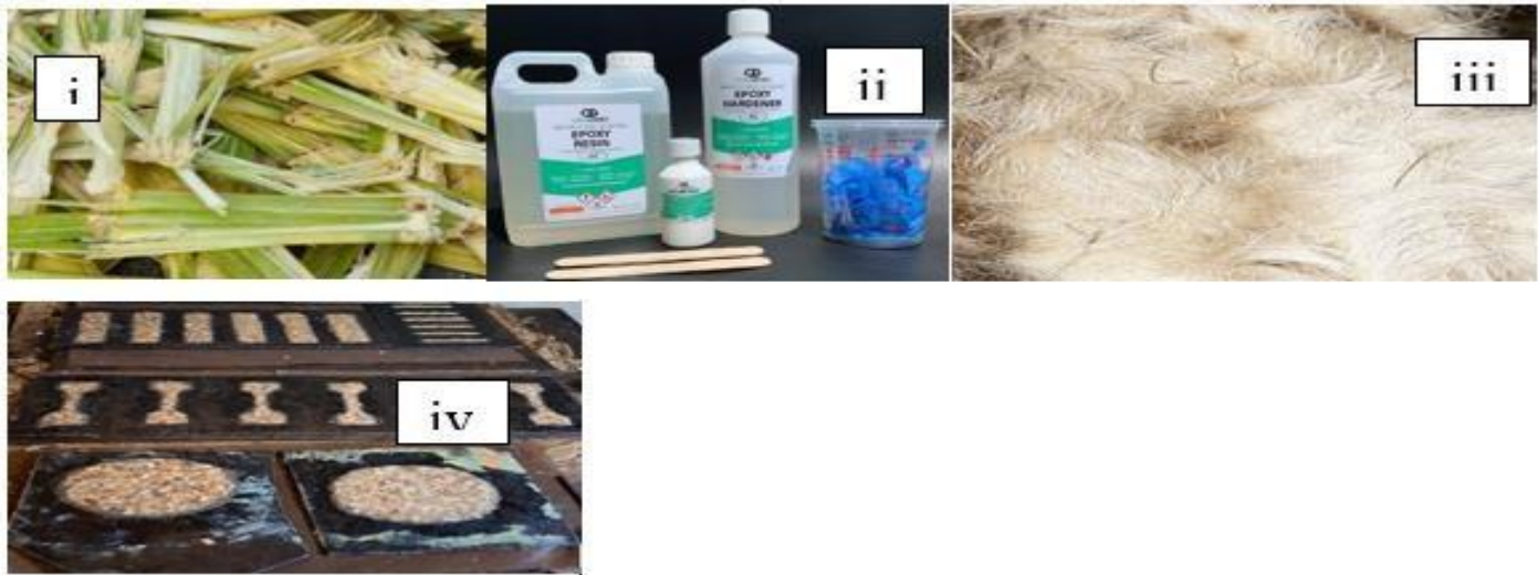
Figure 1: Sugarcane bagasse:(i). Epoxy resin and hardener (ii). Cow hair (iii). Cow bone (iv). Cow bone particulate
